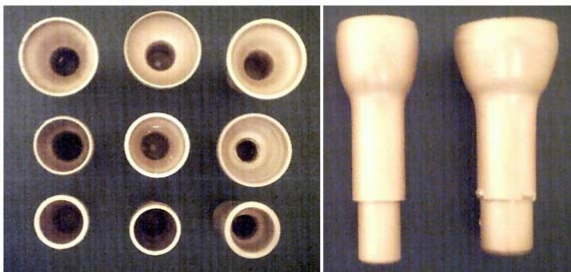
Figure 10. Widened tube ends profile: Top and side view.
