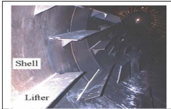
Figure 3. The inside view of a normal rotary dryer.
